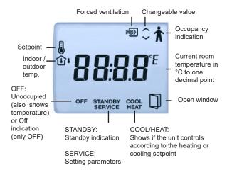
The buttons on the controller enables easy setting of parameter values using a parameter menu shown in the display. The parameter values are changed with the INCREASE and DECREASE buttons and changes confirmed with the occupancy button.
