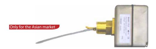
FLS304 is a heavy duty flow switch which interrupts the electric control circuit of the boiler/chiller when there is insufficient water circulation in the boiler/chiller pipe owing to some abnormal condition. The FLS304 flow switch is operated by an electrical blade-type tripping device (stainless steel blade) and can be installed on pipework from 1" to 8" in diameter.
