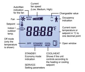
The display is handled using the buttons on the thermostat:
