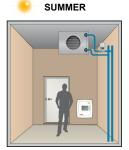
In 4-pipe installations, there are two separate water systems for heating and cooling with separate valves. The thermostat uses two outputs for control of heating and cooling in sequence.
