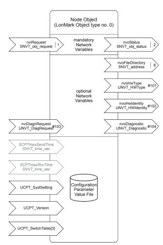
Fig. 6. Profile of LonMark node object
