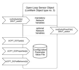
Fig. 9. Profile of LonMark actuator objects for relays
