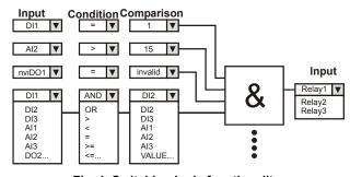
Fig. 1. Switching logic functionality
