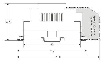
Fig. 10. Excel Smart I/O Compact (dimensions in mm)
