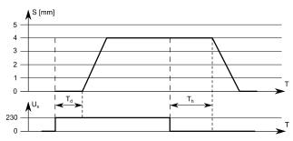
S = stroke $U_s = supply voltage$   $T_d$  = dead time  $T_h$  = hold time
