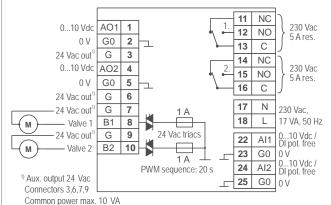
**IMPORTANT:** When the relay outputs are used with 230 Vac voltage, the outputs must be equipped with a fast fuse (max 5 A) that is in accordance with the standard IEC 60127-2.
