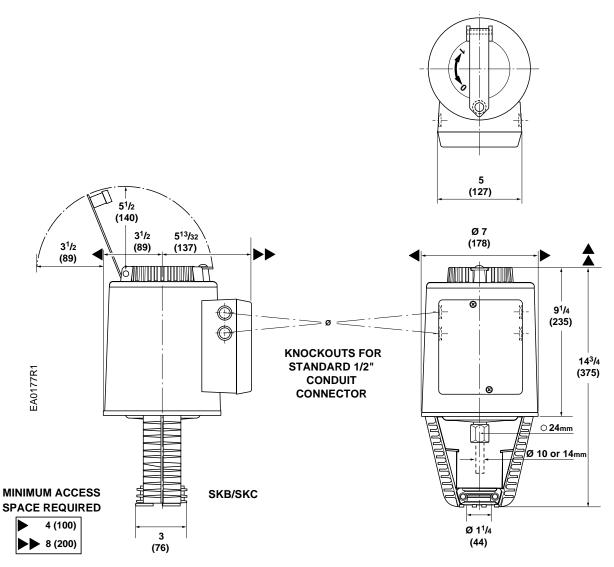
Figure 32. SKB/SKC Dimensions in Inches (mm).
