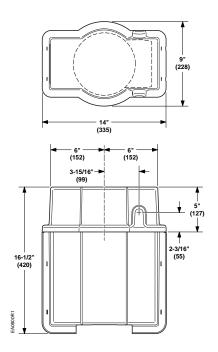
Figure 31. SKB\C Weather Shield, 599-10065 in Inches (mm).
