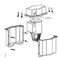
Figure 2. SKB\C Weather Shield.
