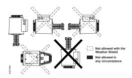
Figure 1. Acceptable Mounting Positions.
