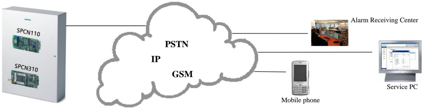
The SPC panels offer multi-path communications via IP, GSM and PSTN. All the modems modules are pluggable to allow any combination to be used. The panel supports remote connectivity over all communication options, to provide engineering functions including configuration or diagnostics, and to the user the ability to remotely manage the premises.
