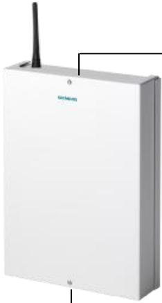
The signals of Intrunet wireless detectors and remote controls can be received via any of the connected wireless access points allowing optimal signal reception and range extension within an application. And the rollout is done very quickly via keypad, web browser or the SPC Pro programming tool.
