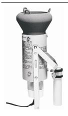
This detector tester contains a hot air generator. For the performance check, the tester is pushed over the detector. The hot air released heats the detector and so actuates an alarm.
