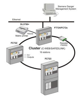
Using a fiber-optic Backbone (C-WEB/LAN) up to 14 of the above mentioned clusters (with up to 16 stations each) can be networked. The entire network may contain up to 64 stations.
