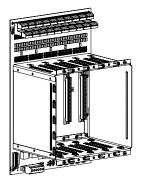
The card cage (5 slots) is suitable for holding a maximum of 5 module bus cards or I/O cards. The card cage is mounted on the carrier (19", card cage) FHA2023-A1. A maximum of two card cages can be mounted on the carrier.
