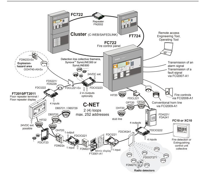
Up to 32 control panels and terminals can be linked to form a cluster (C-WEB/SAFEDLINK network). If the cluster is connected to a danger management system via BACnet, up to 16 control panels and terminals can be networked.
