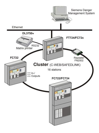
An optical Ethernet network (C-WEB/LAN) allows up to 14 clusters with up to 16 stations to be operated on one network. A maximum of 64 stations is supported in total.
