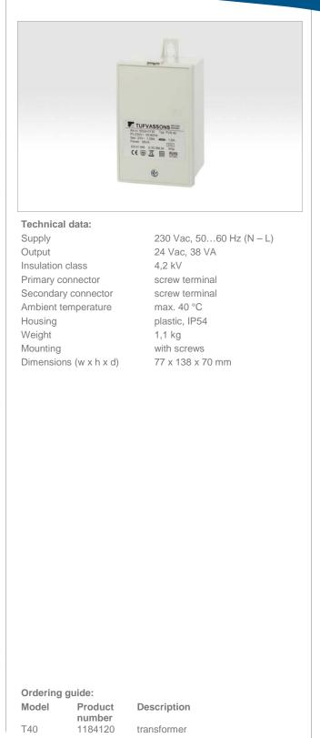
Products fullfil the requirements of directive 2004/108/EC and are in accordance with the following standards. Emission: EN61000-6-3, EN61000-6-4, IEC 62041. Immunity: EN61000-6-1, EN61000-6-2, IEC 62042. Security: EN 61558-1; EN 61558-2-6
