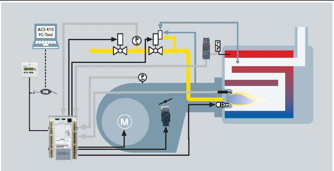
The diagram shows the full scope of functions of the LME7... system. The correct functions are to be determined based on the respective execution/configuration.
