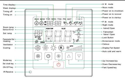
Setting parameter No. 13, the selection of the fan coil system has to be done. 2-pipe or 4-pipe systems can be selected.
