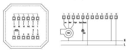
LCF Touch Standard –wiring diagram for 4-pipe fan coil
