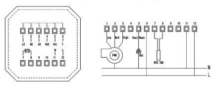
LCF Touch Standard - Manual mode wiring diagram for 2-pipe fan coil
