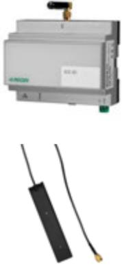
CLO-3G is a package consisting of a 3G modem with a factory-installed SIM card, ready for immediate connection to CLOUDigo. The modem functions as a gateway between a TCP/IP connected Corrigo and CLOUDigo. It has a built-in DHCP function that handles connecting to an external unit.
