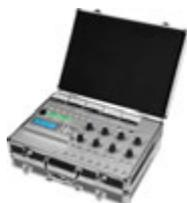
Complete case with everything you need to test Corrigo. Simply plug the controller into the wall socket using the included transformer in order to make simulations, trigger alarms, view indications, etc.
