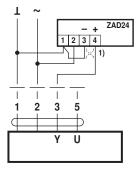
Control with 4...20 mA via external resistor
