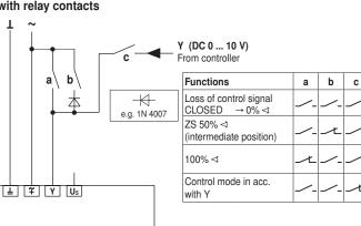
Override control with AC 24 V with rotary control switch
