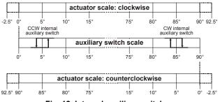
Fig. 12. Internal auxiliary switches
