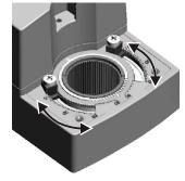
Fig. 10. Mechanical end limits
