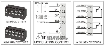
NOTE: Internal auxiliary switches S1 and S4 must be connected to the same power source.
