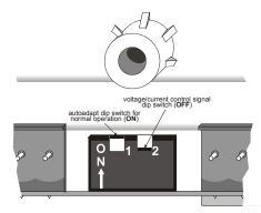
Fig. 7. Dip switches (view with PCB at bottom)
