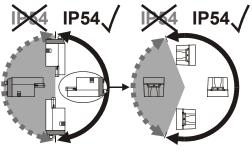
Fig. 13. Mounting for IP54
