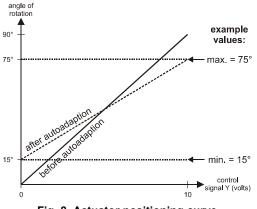
Fig. 8. Actuator positioning curve
