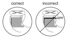
Fig. 11. Correct / incorrect tightening of end limits
