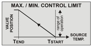
Fig. 2. Minimum Heating Example
