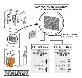
Fig. 13. LonWorks® connection and termination module
